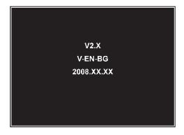
Initially, the DVR will boot-up and display the current version and release date of the DVR firmware for a few seconds.
